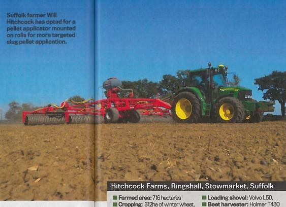
Over the weighbridge it tips the scales at 10.2 tonnes and that hefty weight means the roller can be employed as a cheap secondary cultivator, used by the Hitchcocks on lighter land behind a disc/tine cultivator to produce a seedbed ahead of the farm's power-harrow
