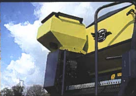
The drill itself comprises three hoppers — two main ones and a mini-hopper at the front.
