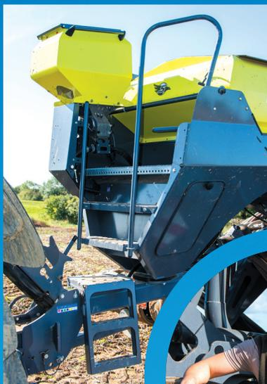
Above: Access to the three tanks is safe and simple thanks to this set of tapered steps and guard rails
