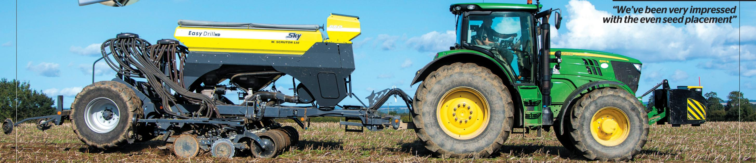
► coulter and this can be biased either towards the front press wheels or rear closing wheels to suit the type of crop being drilled, soil type and conditions.
