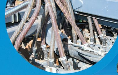
Above inset: An adjustable weight transfer system exerts up to 250kg of pressure on the coulters or the press wheels
