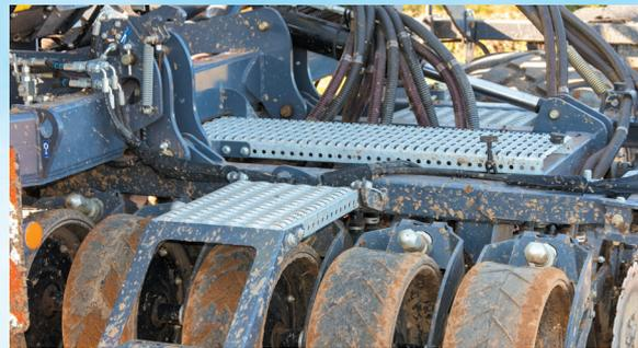
Above: The drill's depth is adjusted using a turnbuckle system fitted above the front press wheels
