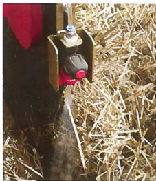
Running directly behind the subsoiler legs, the NitroJet nozzles apply fertiliser in the narrow band where the seed is placed.
