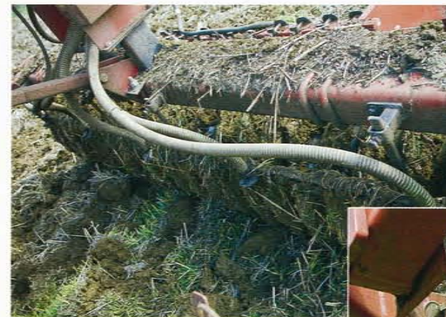
The subsoiler band sows the rape seed into 60cm wide strips above the loosened soil.
