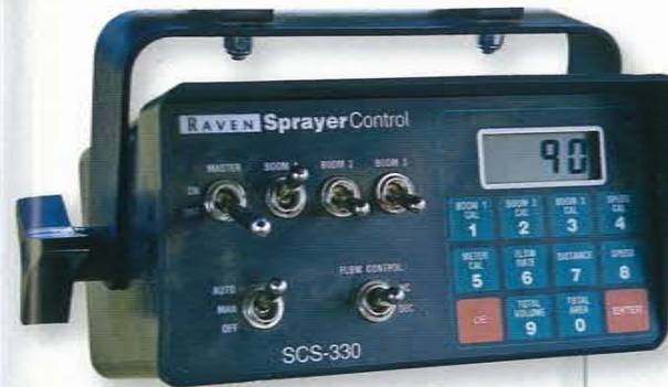
The in-cab control box enables the operator to alter the liquid fertiliser rate on the move.
