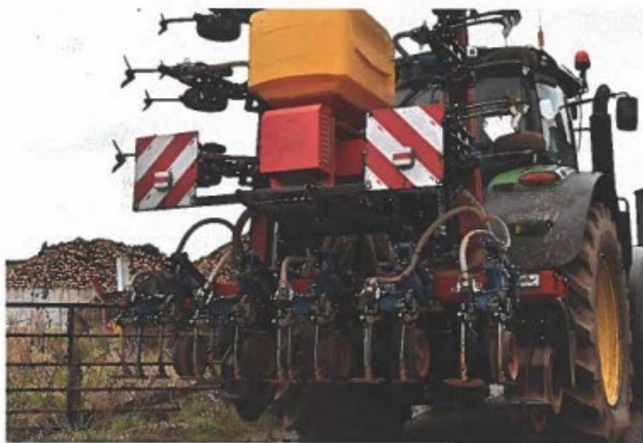
A 12-row, 6m inter-row cultivator, set at 50cm spacings, arrived at Gillow Farm last spring.
