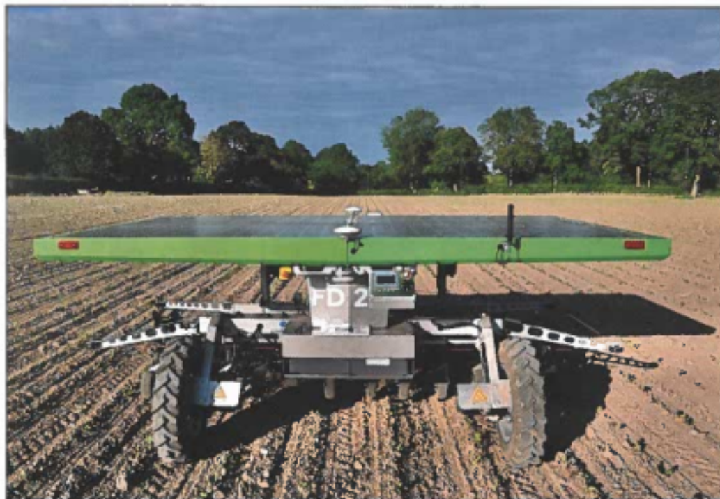
A large solar panel on top of the FarmDroid provides energy to both drill and then hoe the beet, guided by GPS.
