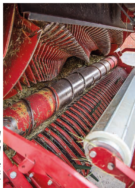
Plastic tines on the Flex-Load pick-up make it unique. The tines taper from 20mm to about 10mm thick, rake very quietly and can be quickly changed by opening the clamping screws behind the deflector plate.
