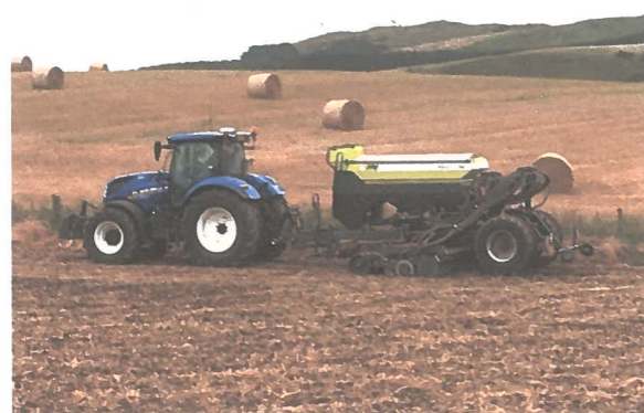
ABOVE David uses a Sky EasyDrill for the majority of the drilling, with three hoppers to apply fertiliser and micro-granules simultaneously
